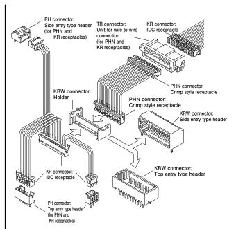
With the JST standard product KR connector as the core, according to using multi-harness insulation displacement connection by an automatic IDC machine, a holder for making a dual-row socket, a corresponding dual-row header, a header for wire-to-wire connection and so on, the high-density mounting of harnesses such as complicated shape is enabled.
