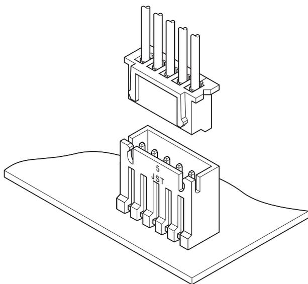
This is a XH connector high-box type with a mounting height of 17.0 mm and a thickness of 5.8 mm. It provides stable state contact even for micro-voltage and current circuits.
