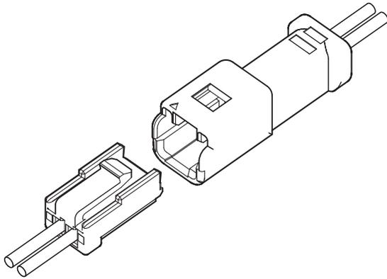
This is a small-sized, wire-to-wire, single row connector at 1.5mm pitch. It is not only compact for applications with limited space, but also provides a clear mating and locking sensation upon connecting the plug and receptacle.
