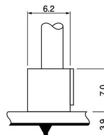
Note: 1. Tolerances are non-cumulative:  $\pm 0.05\text{mm}$  for all centers. For connectors with 5 or more circuits the hole dimensions will differ from the above values. Contact JST for details.
