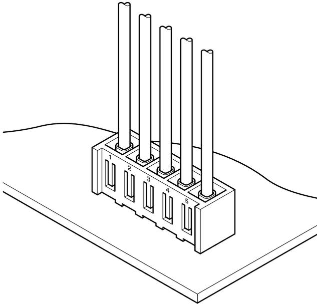
The SDN connector is a 3.96mm pitch board-in crimp style connector capable of connecting a wide variety of circuits including signal and power supply circuits. The connector features a slim, low-profile design. In addition, it has an exclusive lance construction to reduce insertion force, thus substantially improving the working efficiency in mounting the contact.
