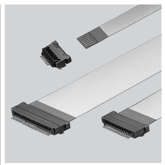
The FPZ is a Zero Insertion Force (ZIF) connector designed for surface mounting of FFCs with a lead pitch of 1.0mm. With its mating slider serving as a guide, the FPZ connector ensures easy and reliable connection. It also features high heat resistance, which is suitable for surface mounting, and can be supplied in the form of emboss taping to facilitate automatic mounting.
