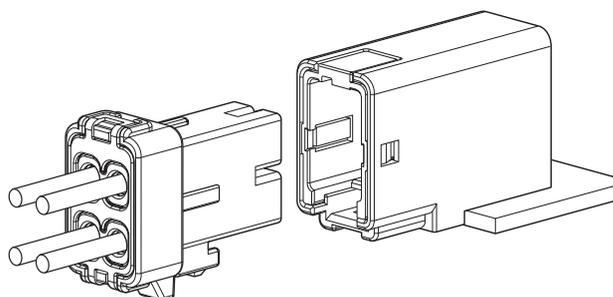
This JWPS connector can be used for the place of which especially waterproof is required.
