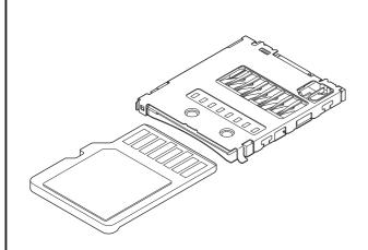
This is the connector for micro SD card in which mounting height of 1.45 mm maximum is kept and push-push mechanism is adopted.
