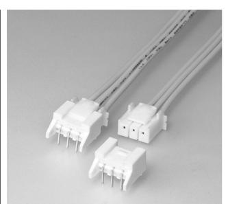
VU connector is small type 3.96mm pitch PC board connector for large current and has the high reliability in a power supply circuit, considering the fully shrouded connector header structure against "vibrating connector" and "distorted extraction".
