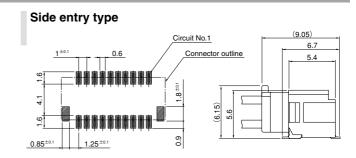
Note: 1.The above figure is the figure viewed from the connector mounting side. 2.Tolerances are non-cumulative: ±0.1 mm for all centers.
