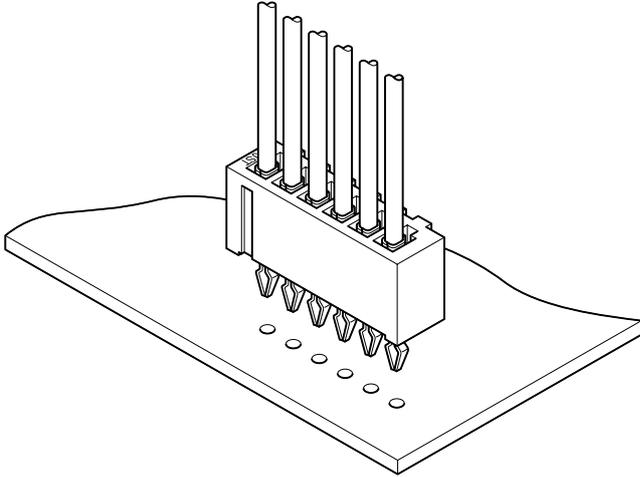
**This 2.5mm pitch multi-circuit board-in connector meets the needs for high-density mounting on printed circuit boards efficiently and economically. The connector can be used for VCRs, car stereo systems, audio products, and many other consumer-oriented electronic products.**
