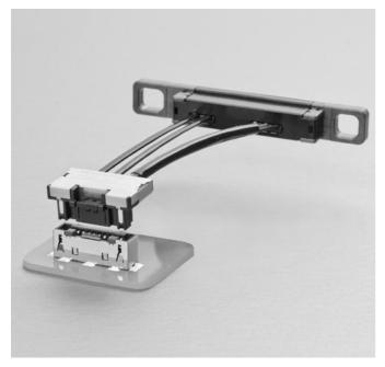
This AS connector consists of the female connector on PCB side and the high-speed differential transmission harness used for internal connection between the PCB and the HDD corresponding to SATA standard for automobile equipment such as HDD navigation system.
