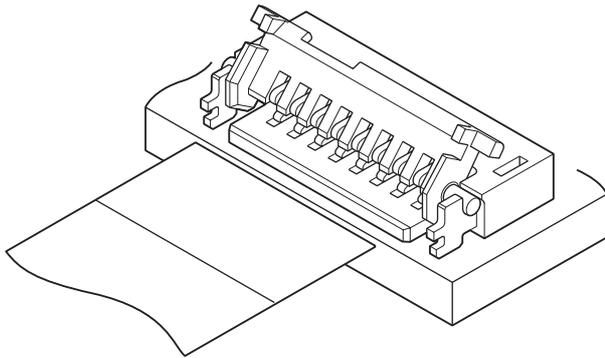
**FHS connector is a space-saving type connector for FPC with 3.1mm depth, though it is low profile of 0.9mm mounting height. 0.2mm thick standard FPC.**
