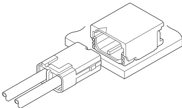
**This low profile type connector with height of 3.0mm is designed for connection to stroboscope flash and realized space saving.**
