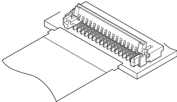
**In addition to achieving space saving and low profile features demanded by the market, this connector also realizes superb operability by adopting a FPC with protrusion. The use of the FPC provides secure and foolproof mating at the customers' production site.**
