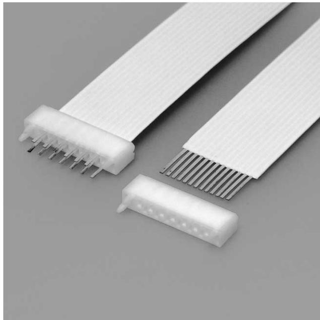
**This board-in type connector provides direct soldering connection between the conductor part of the 1.0mm pitch FFC and the PC board.**
