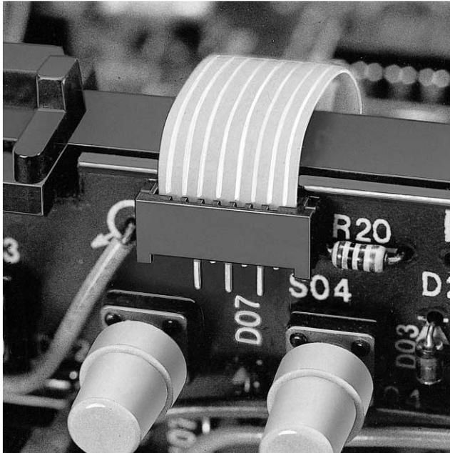
The FM connector, a miniature connector with a thickness of only 3.0mm, was developed to connect flexible flat cables (FFC) or flexible printed circuits (FPC) with a lead pitch of 1.0mm to printed circuit boards. It is ideally suited for connections inside high-density equipment or between mechanical units. The contact is constructed to ensure a stable connection and high reliability even under vibration and impact. Connection is easy with a simple snap-in action.
