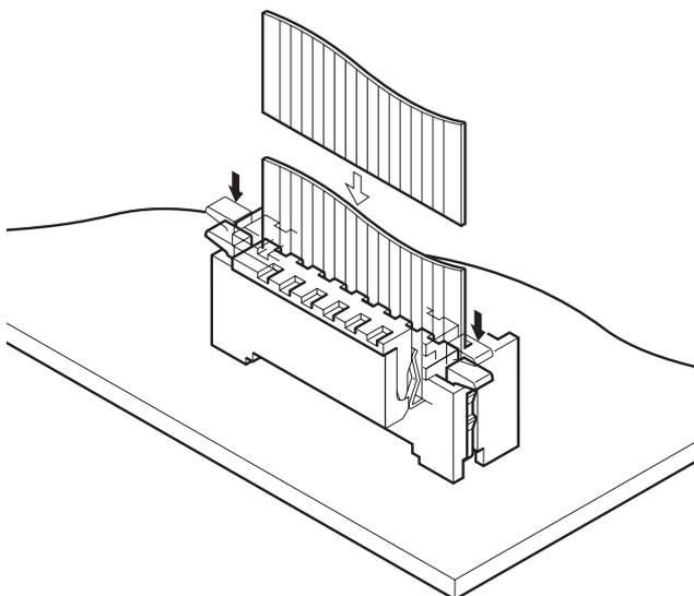
**The FDZ connector, a Zero Insertion Force (ZIF) connector, was developed to connect FPC and membrane switch leads. This combination of features allows greater freedom in internal wiring designs. No force is required to insert the leads. Once inserted, the leads are securely held and locked by moving the slide. The contact is double-sided to ensure greater reliability.**
