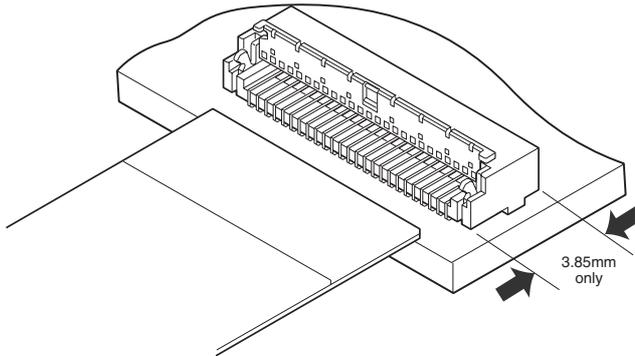
**Space saving flip lock type connector, with 1.8mm height and 3.85mm depth.**
