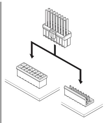
The reliable XL connectors have been developed by utilizing the technology of JST's field proven VH and SM connectors. The XL connectors are being used in electric appliances, vending machines, and office automation equipment.
