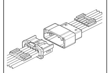
This connector is a 2.5mm pitch wire-towire connector, having incomplete mating prevention mechanism. 2-circuit and 3circuit connectors have control key to prevent connector from mating with incorrect circuits, thus, several same circuit connectors can be used.
