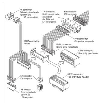
Based upon JST's field proven KR series connectors, the KR series family of connectors have been expanded to meet the requirements of high density packaging. The KRW connector allows double-row wire-to-board connection using either the KR or PHN connectors. Whilst the TR connector allows wire-to-wire connection. also using either the KR or PHN connectors.
