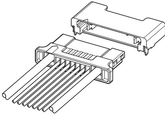
This connector is for connecting the lithium polymer battery or for connecting DC-IN, and has the sequence structure for connection to the power supply circuit in preference to connection to the signal circuit by dividing the signal circuit and power supply circuit clearly. Moreover, this is the low profile connector (space saving) for applying the high current by adopting the heat radiation structure.
