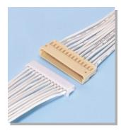
This 1.5 mm pitch wire-to-wire connector is a compact, space-saving interconnect that mates with both crimp and IDC sockets. The four-sided box housing structure is resistant to mechanical stress and misalignment which can cause irregular external forces during the insertion and withdrawal process.
