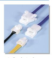
This is a plug type crimp style connector for wire-to-wire in the 2.0 mm pitch PA family connectors with secure locking device. It is applicable for mating with both crimp and insulation displacement style PAF connector socket. Two types connector such as a panel lock with retainer mountable type and a free hanging type can be prepared.
