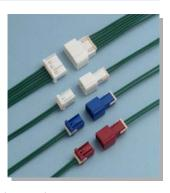
This connector is a 2.5mm pitch wire-to-wire connector, having incomplete mating prevention mechanism. 2-circuit and 3-circuit connectors have control key to prevent connector from mating with incorrect circuits, thus, several same circuit connectors can be used.
