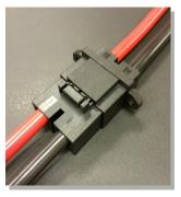
This connector is corresponding to large current up to 50 A with single circuit (when using AWG #8). The 4 and 6 circuits of the J5200 series Dual-row type can select either the bulk insertion of the receptacle housing or the module types.
