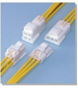
The YLN connector adds variation in shape to the existing color variations of the YL connector in order to improve identification of connectors. Moreover, this connector has a mechanism to prevent incomplete mating by utilizing the inertia force generated when the plug and receptacle are mated and therefore, ensures complete mating.
