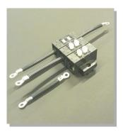
This is a short circuit type power supply system wire-to-wire connector that is configurable up to 4 lines. For example, for one line on the input side, the output side can be branched into 1 to 3 lines according to a use application. It is also possible to its reverse. Use by mounting the crimped ring tongue terminal R8-5.
