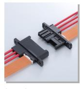
In unit connection, this RIZ connector is a hybrid type connector with combined signal and power supply circuits, absorbs misalignment between units, and excels durability. \*Pitch for signal circuits is 1.5mm. Single row realizes slim design 9.0mm and space reducing.
