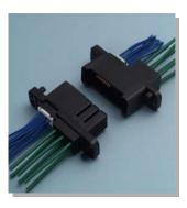
This connector is a hybrid type double-row drawer connector combined signal and power supply circuits connector to connect the units. RWZ connector with lever locking device is adopted as applicable socket to prevent incomplete mating.
