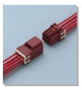
This HIL connector is 3.3mm pitch wire-to-wire connector that has a mechanism to prevent an incomplete mating when mating connector.
