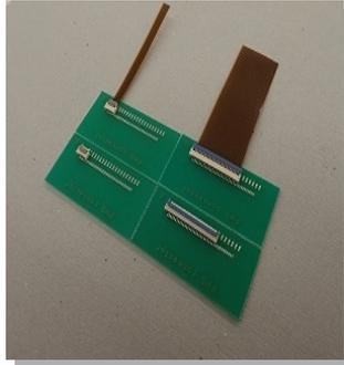
This ZIF type 'flip lock' FPC connector achieves a low-profile feature of a 0.9mm mounting height despite the thickness of the FPC being 0.3mm.
