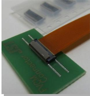
This FVCM connector is the first mid-flip type 0.2 mm pitch connector for FPC in the connector industry. It is designed for the use of multipolarization, operability and both upper and lower contacts. Moreover, it inherits from tilt type, and it improves the freedom of design for placing at the PC board dramatically.
