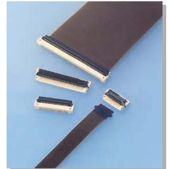
This connector for the 0.3mm thickness FPC with a mounting height of 1.3mm. FPC with protrusion prevents incomplete insertion and mis-insertion, so that it provides reliable connection.
