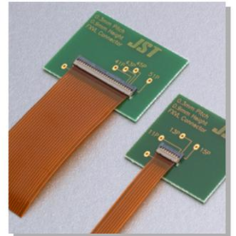
This FXVL connector is a space saving and low profile connector for FPC demanded from the market, and realizes 0.3mm pitch connector with a mounting height of 0.9mm and depth of 2.68mm. In 0.3mm pitch FPC connector, the smallest product in mounting area on the board has been provided.
