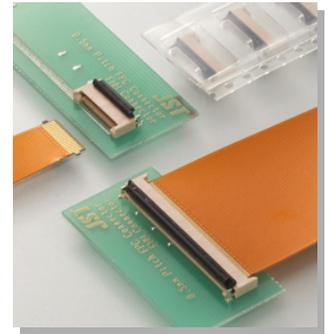
This is connector with the double-sided contact for FPC. As FPC with protrusions is used for this FHH connector, prevention of incomplete insertion and mis-insertion are realized and connection reliability is improved.
