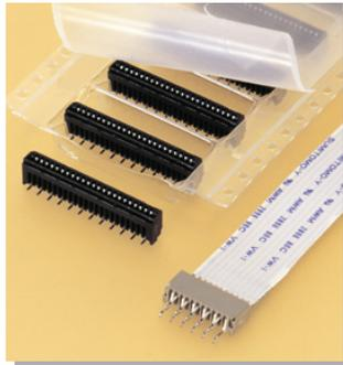
This connector is 1.0 mm pitch for FFC connection. Realized low cost multi-core by adopting contact structure on one side. In addition, it is a multi-entry type connector that has both DIP and SMT types.
