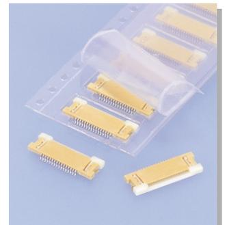
This is a 0.5 mm pitch FPC connector with a mounting height of 1.2 mm, compatible with standard FPCs with a terminal (lead) thickness of 0.3 mm. This connector features a Zero Insertion Force (ZIF) connection to effectively extend the lifespan of FPCs by reducing wear during mating and unmating.
