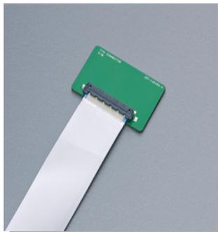
This is 0.5mm pitch connector for FPC which has the exclusive GND contact and enables high-speed transmission with connecting to the impedance controlled FPC. Adopting the auto lock mechanism that makes lock by performing the one action of snap-in-work, the workability improvement is realized.
