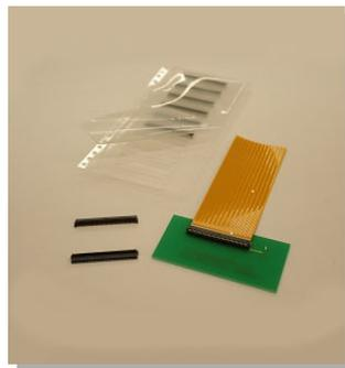
This is 0.5 mm pitch, back flip type FPC connector for 0.3 mm thick FPC. Realized space saving with thin of 1.0 mm mounting height. Considering the transmission of various high-speed interfaces such as Thunderbolt<sup>TM</sup>, the differential impedance shall be matched at 90Ω.
