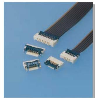
FHS connector is a space-saving type connector for FPC with 3.1mm depth, though it is low profile of 0.9mm mounting height. 0.2mm thick standard FPC.
