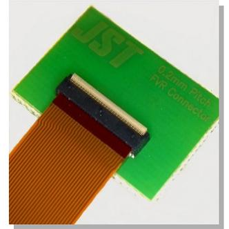
This is low profile and space saving type connector for FPC with 0.2 mm pitch, 0.95 mm height, and 3.0 mm depth. Back flip type of double-sided contact improves the freedom for routing of FPC.
