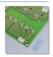
This contact can be placed anywhere on a PC board. This makes it flexible to connect with other male components with different pitches and different numbers of pins. The receptacle is mainly designed inside the PC board thickness to have a low profile connector.
