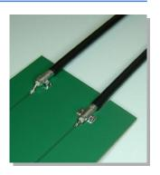
This is a terminal to fix a coaxial cable to the PC board. By press-fitting the dimple on the terminal foot portion into the PC board, the terminal is fixed when installing it onto the PC board and the soldering work is improved.
