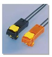
This connector for air-bag has intelligent CPA, which allows locking the connector, incomplete mating detection and release of short-circuit at the same time.
