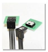
Smallest SMT connector in the world which can be used in automotive application (Height: 3.5mm)
