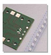
This contact can be placed anywhere on a PCB. This makes it flexible to connect with other male components with different pitches and different numbers of pins. The receptable is designed inside the PCB thickness. This makes is possible to have reflow processes on both sides if the PCB without damaging the SBO contact.
