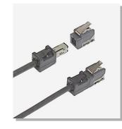
This is compact high-frequency signal connector with enhanced GND performance, suitable for in-vehicle equipment with antenna communication (GPS, ETC/DSRC, Wi-Fi, Bluetooth). It is also suitable for coaxial video signal transmission in combination with cable-side connectors for noise suppression. It is surface mount technology (SMT) compatible products.
