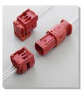
Compliant with the ISO 19689, 0.64 mm individual waterproof, 6 pole wire to wire connection connector. The retainer is a pre-set type for both female and male housing. Protection cover to female connector from water and dust is selectable to the installation direction.
