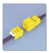
0.64 unsealed wire-to-wire connector with CPA and shorting bar mechanisms for Air-bag application. Providing Connector Position Assurance, positive mating and completion of circuit in one pressing motion.
