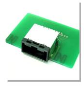
This HIE connector complies with HDMI E Type for automobile equipment such as navigation system.
