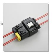
0.64 mm mat sealed wire to wire connector with rigid design and spring lock mechanism. Spring force prevents half-mating during mating and keeps constant rigid connection between male and female connector.
