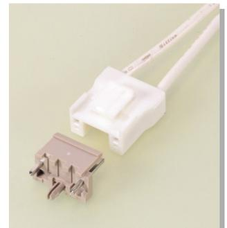
Can be connected to vinyl insulated flat cables (such as SPT, HVFF) ranging from AWG #20 to 16 which are used for primary sides of power circuits.
