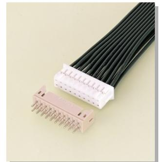
This is a 2.0 mm pitch dual-row wire-to-board connector. With a mounting height of 8.8 mm and a depth of 5 mm, the low-profile, space-saving design supports the miniaturization and high-density design of devices.
