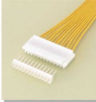
This is a 2.5 mm pitch connector for connecting PC boards and wires, and consists of a contact, housing and header. There are three types of Header: top, side and bottom entry types, which allow wires to be drawn up, down, or parallel to the PC board by combining them.
