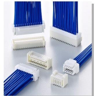
This is a wire-to-board connector with 1.5 mm pitch, dual-row structure and secure lock mechanism for high-density board designs. Low insertion force and good insertion feeling ensure reliable mating operations.
