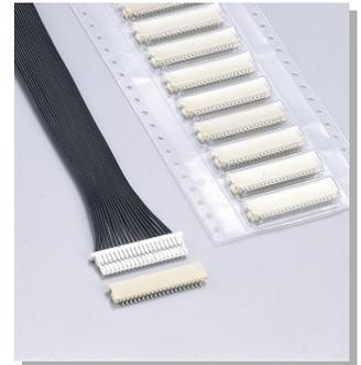
This is an ultra-thin 1.0 mm pitch wire-to-board connector for thinner and smaller devices, with a mounting height of 1.8 mm for the normal type and 1.4 mm for the offset type.
