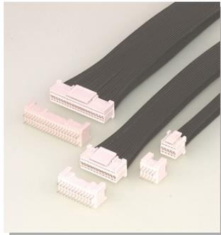
This wire-to-board connector features a robust locking system that is not only easy to work with, but also provides adequate durability to irregular outside force. The 2.0 mm pitch, dual-row design is suitable for high-density PCBs used in electronic equipment.
