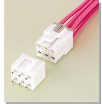
This VL connector is 6.2 mm pitch wire-to-wire and wire-to-board connector, designed for large current. Secondary retainer, which prevents from insufficient insertion of contact and coming off contact, may use and large current circuit can be connected certainly and safety.
