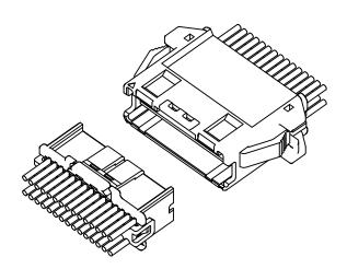
This is the 1.5 mm pitch dual-row type wire-to-wire connector with secure locking device that is correspondent to the high-density equipment design. A good mating feel makes the occurrence of incomplete mating suppressed.
